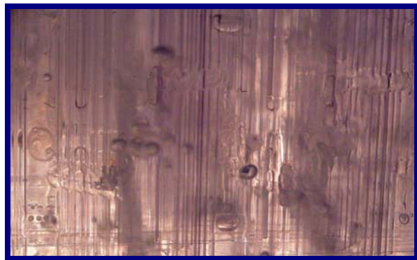
(b) Large slug air bubbles formed in the VF media at an air flow rate of 3.0 SCFM/ft 2
