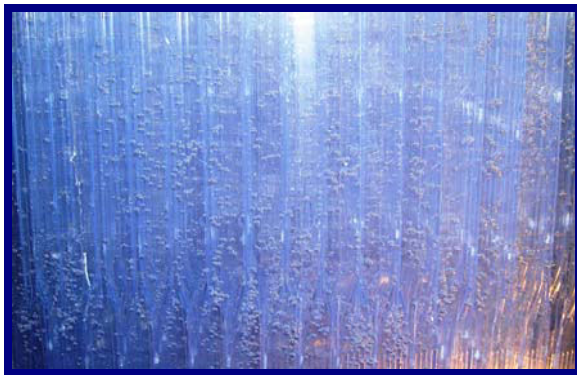
(a) Small air bubbles in the VF media at an air flow rate of 1.0 SCFM/ft 2
