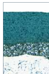
Cross section of Flygt epoxy coating
