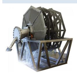
The new model eliminates rubber seals, roller chain and sprockets, internal bushings and bearings for less maintenance
