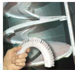
Durable segmented brushes make replacement easy.
