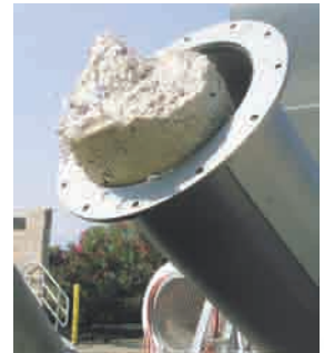
The discharged solids are cleaned and compacted.
