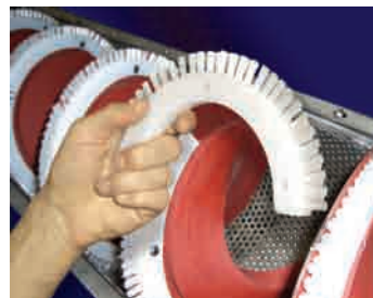
Segmented nylon brushes offer high strength and convenience.
